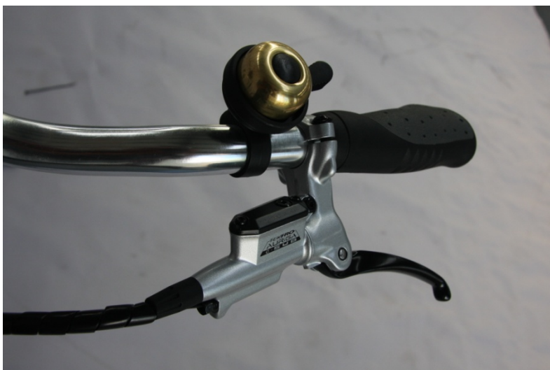
Tektro Auriga E-sub hydraulic brake lever with electric cut off function.
