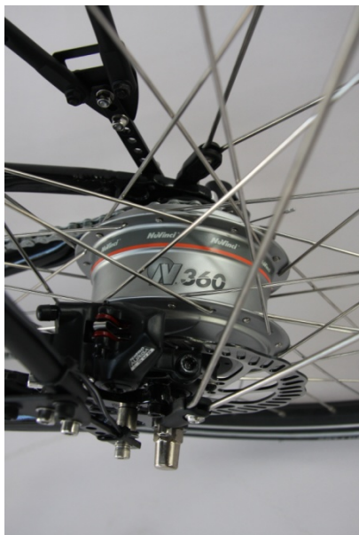
NuVinci N 360 hub And hydraulic disc brakes.
